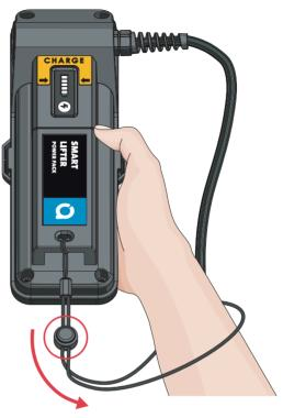
4. Wear the wrist strap and adjust the toggle to tighten it. Hold the Power Pack securely at all times and DO NOT release it.
