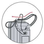
2. Once the loop is fully threaded, expand it and pass the strap through the opening.
