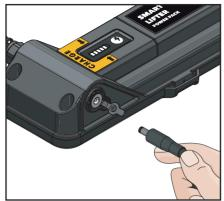
5. INSERT THE CHARGING PLUG Insert the plug into the Power Pack's charging port. Ensure the Power Pack is placed in a well-ventilated area, away from direct sunlight.
