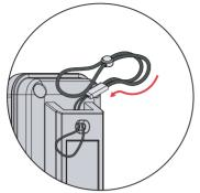
1. Insert the thin loop of the wrist strap through the slot on the back of the Power Pack.
