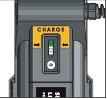
2. ASSESS THE LED GAUGE If the LED gauge displays only two GREEN bars, remove the Power Pack from the vehicle and charge it immediately. **DO NOT** use the Power Pack when the charge level is at two bars.
